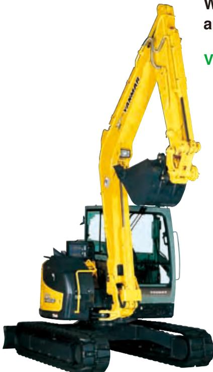
The ViO80 is equipped with a direct fuel-injection engine that complies with Japanese non-road special motor vehicle emission regulations, U.S. EPA intermediate Tier-4 emission regulations, and Euro 3A regulations, making it compliant with the latest regulations in Japan, the U.S. and Europe.
