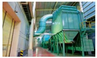
Dust collector installed inside the factory building
