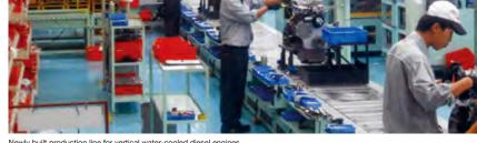
Newly built production line for vertical water-cooled diesel engines
