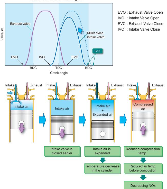
Intake/exhaust valve lift diagram
