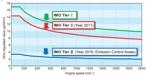
The regulations on NOx and SOx emissions continue to grow stricter. In special "Emission Control Areas" established by various countries, the sulphur content of fuel oil used must be 0.1% or below after 2015. The limit of 0.1% sulphur content in fuel oil has already been in effect within the EU for vessels anchoring within a bay or traversing inland waterways since January 1, 2010.
