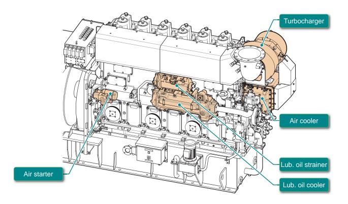
Modular construction of the turbocharger and air cooler Modular construction of the lub. oil system
